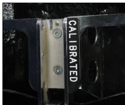
Figure 25: Calibrated Torso angle measurement surface block attached to trunk of weight hanger arm.
