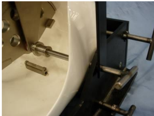
Figure 20: H-Point locator bars installed through vertical support rods, jig side and H-PM H-Point location.
